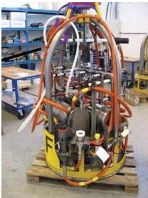
Figure 6-4 Example of large passive acoustic detector prepared for installation (left) and compact passive acoustic detector installed on a topside valve (right).
